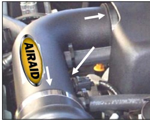
**11.** Install the 7/16" rubber grommet (#15) into the Airaid Intake Tube (#2). Insert the factory AIT sensor into the grommet. Slip the Airaid Intake Tube into the urethane hump and reducer hoses. Align for best fit and tighten the remaining hose clamps. Tighten the MAF bracket and reconnect the AIT sensor wiring harness. Apply the Airaid Bubble Decal onto the Intake Tube as shown.
