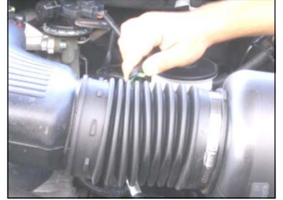
**3.** Remove the crankcase breather hose from the factory intake tube and the valve cover. Disconnect the Air Intake Temperature (AIT) sensor wiring harness from the sensor. (4.6L Engine only: Disconnect the Idle Air Bypass Valve (IABV) inlet tube from the factory intake tube.) (5.4L Engine only: disconnect the IABV, save the plastic hose for reuse.)
