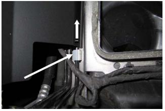
10. Snap the Line Holder (#22) onto the ABS line closest to the panel assembly and remove the adhesive backing. Gently push the Panel away from the line and slide the Line Holder behind the Panel. Relax the Panel, and allow the Adhesive pad to bond the Panel. This will isolate the Panel and prevent contact with the ABS line.
