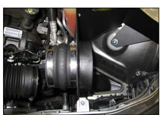
**14.** Install the Hump Hose (#7) and Clamps (#20) onto the Filter Adapter. Leave the Clamps loose for now.
