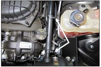
**16.** For 3.6L V6 Pentastar equipped vehicles: Install the Smaller, 5/8" hose (#11) onto the Barbed Fitting and factory hard line. Snap a Speed Clamp (21) on each end of the hose to secure it in place.
