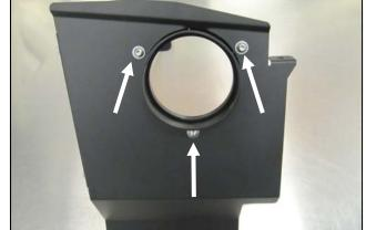
**5.** Install the Filter Adapter (#6) onto the Front Panel as shown using three 1/4-20 Button Head Screws (#12) and 1/4" Flat Washers (#13).
