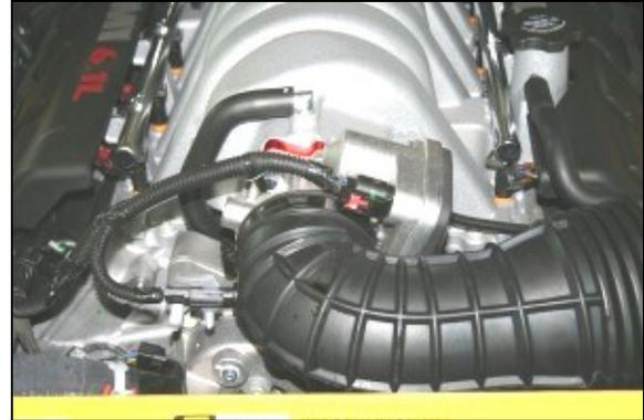
4. Reinstall the factory intake tube, and tighten the hose clamp. Reconnect the Air temperature sensor and throttle body motor. **Re-connect the negative battery cable!**
