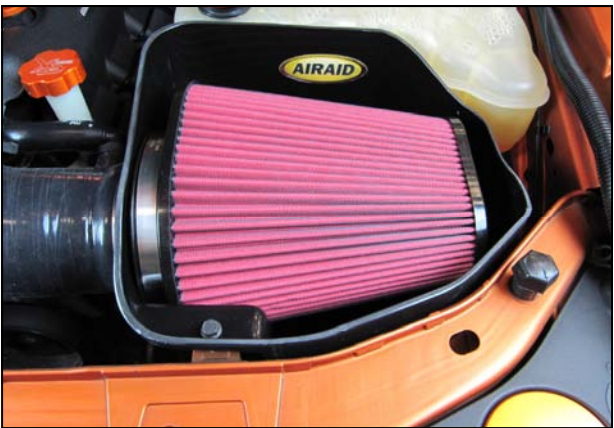
12. Install the Airaid Premium Filter onto the Filter Adapter. Apply the Airaid Bubble Decal inside the Airbox as shown.
