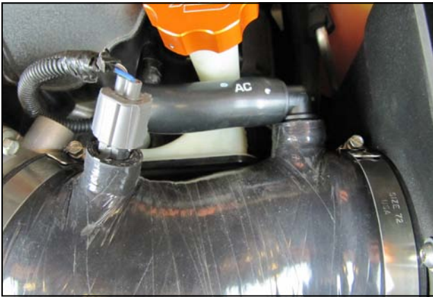
10. Reconnect the air temperature sensor, and the crankcase breather tube to the Barbed Elbow .
