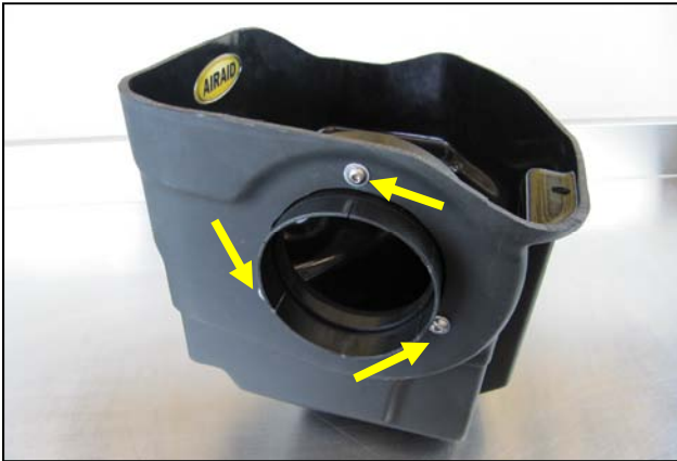
4. Install the Filter Adapter onto the Cool Air Box using the three ¼" Button Head Screws and ¼" Flat Washers, (#s 8&9). Apply the Airaid Bubble Decal inside the Air-box as shown.
