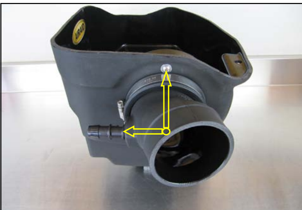
8. Install the Intake Tube into the Coupler as shown, with the Barbed Fitting in the Nine O'clock position. Do no tighten the Clamp at this time.
