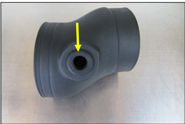
6. Insert the Grommet into the Intake tube.
