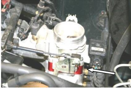
5. Install one gasket (#4) on the intake manifold, then the Poweraid spacer (#1), with the other gasket (#4) on top of it. Next install the throttle body using the four provided 6mmx50mm bolts (#2) and washers (#3), and tighten to manufacturer's specifications.
