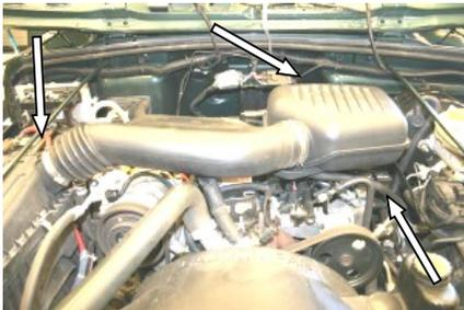
7. Re-connect the intake tube to the airbox, re-connect the breather hose, and tighten all hose clamps.
