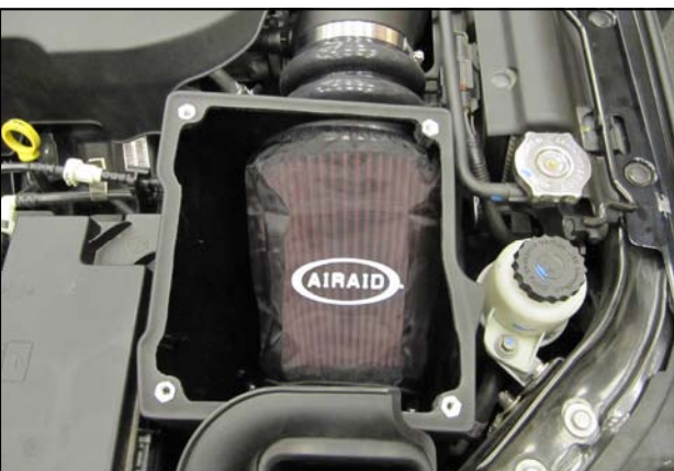
21. Pre Filter Option: Part Number 799-445 For maximum protection in the harshest environments Airaid offers a slip on Pre Filter. - Prolongs Cleaning Intervals - Water Repellant - Free Flowing Protection
