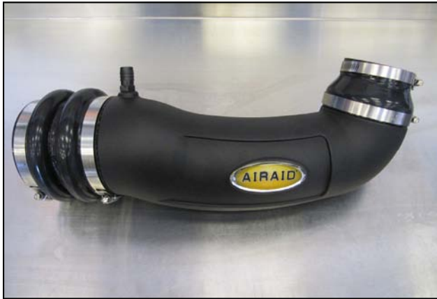
13. Slide the Double Hump Hose , and two #72 Hose Clamps, onto straight end of the Tube. Slide the Silicone Reducer and the #48 and #64 Clamps on the 90 deg. bend of the Intake tube. Leave the Clamps loose for now. Apply the Airaid Decal to the Tube as shown.
