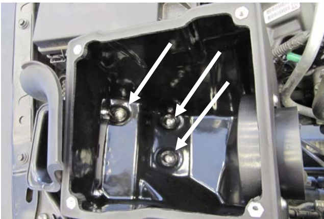
11. Mount the Cold Air Box assembly in the inner fender using the three 3/8" x 1 1/2" Button Head Bolts.
