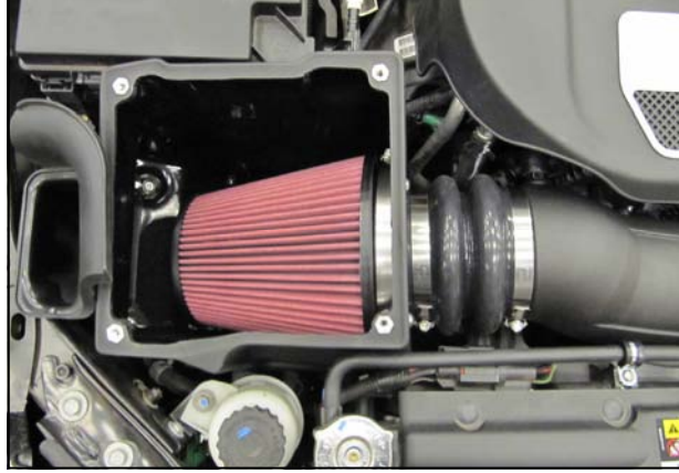
18. Install the Airaid Premium Filter onto the Filter Adapter.
