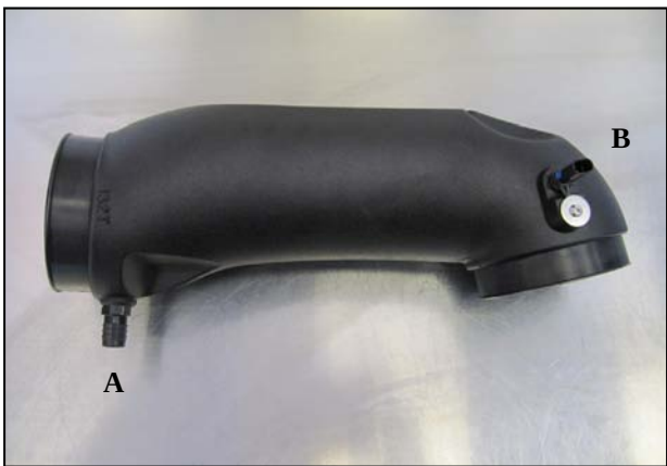
12. A.) Install the 5/8" Barbed Fitting into the threaded 3/8 hole in the side of the Airaid Intake Tube. B.) Transfer the air temp sensor from the factory intake into the Airaid Intake Tube and secure it using the #8-32 x 1/2" Button Head Bolt and #8 Fender Washer.
