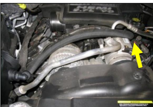
**8. 5.7 Hemi engines only.** Using the supplied straight 3/4" hose, connect both ends to the nylon fitting and oil fill nipple as shown. Fasten both ends using the supplied nylon speed clamps. Adjust the nylon fitting downward to clear the factory intake tube assembly.
