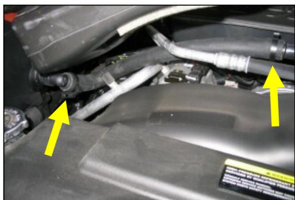
**7. 4.7L engines only.** Using the supplied pre-formed 3/4" hose, connect the nylon fitting to the remaining plastic factory hose as shown. Fasten both ends of the hose using the supplied nylon speed clamps. Adjust the fitting downward to clear the factory intake tube assembly.
