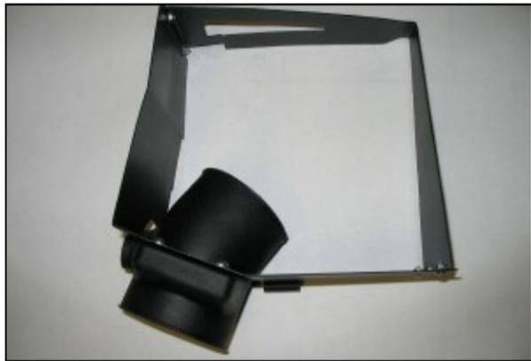
**4.** Using the supplied #6 screws, nuts and washers, assemble the two panels as shown above. Next, install the supplied air filter adapter using the supplied 1/4-20 bolts and washers.
