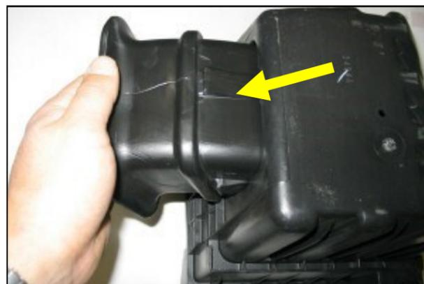
**3.** Using a 13mm socket, remove the air box base from the engine compartment. Using a flat blade screwdriver, carefully unsnap the box inlet from the base and remove it. Reinstall the factory base in the engine compartment without the inlet.
