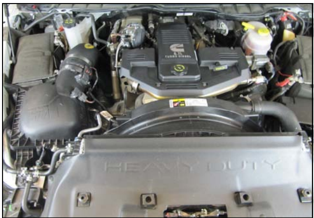
11. Double check your work. Make sure all Clamps are tight and reconnect the negative battery cables.
