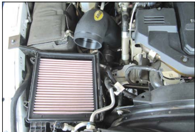
6. If you are installing an Airaid Jr. kit, install the Airaid Premium Filter at this time.
