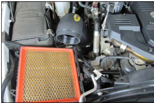
5. Slide the Airaid intake tube into the turbo inlet but leave the clamp loose for now.
