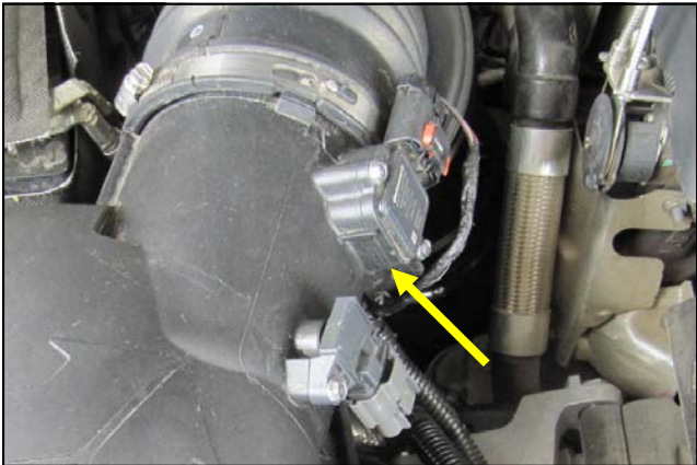
3. Gently pry the harness anchor out of its tab on the airbox and free the wire harness.
