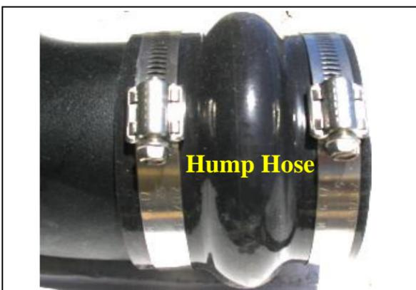
**8.** Install the hump hose and coupler provided onto the Airaid MIT with the supplied hose clamps. The straight coupler is positioned on the throttle body end and the hump hose is positioned on the air filter end.
