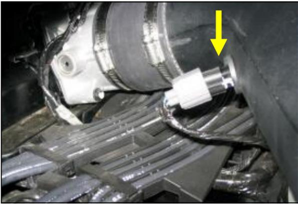
10. Reconnect electrical connector on factory air temperature sensor.
