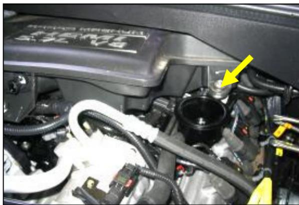
**4.** Remove oil fill cap from valve cover. Using 10mm socket, loosen two factory housing bolts. Remove housing from engine.
