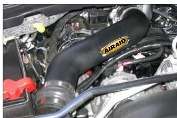
**9.** Check for any foreign objects or debris in the intake path & install Airaid MIT assembly on engine. (*Note: Leave hose clamps loose until final assembly*) Apply the Airaid Bubble Decal onto the Intake Tube as shown.
