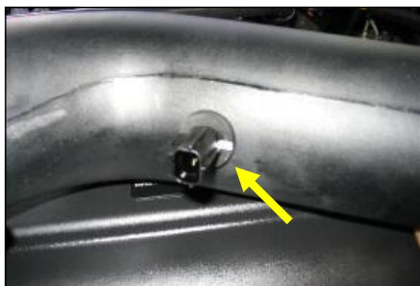
**7.** Install the supplied grommet and factory air temperature sensor into the Airaid MIT.
