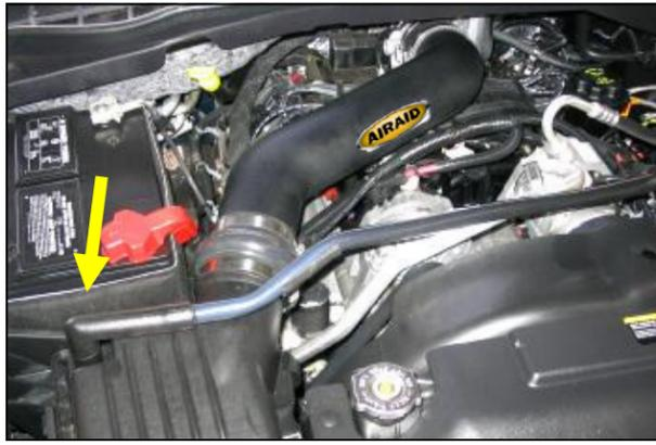
11. Adjust hose assembly for final position and tighten all four hose clamps. Reconnect valve cover breather hose to air box lid and replace oil fill cap.
