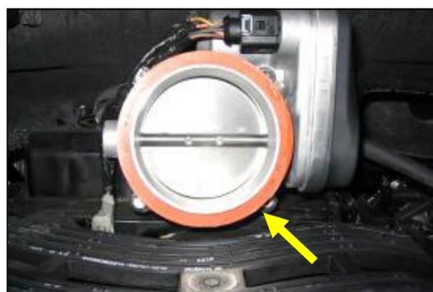
**6.** Remove factory orange seal from throttle body.
