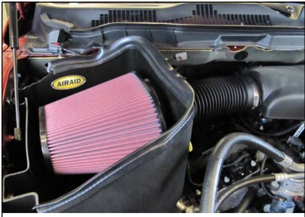
12. Install the Airaid Premium Filter onto the Filter Adapter inside the Cool Air Box. Install the Weatherstrip onto the Cool Air Box as shown, with the contour rolling away from the Filter. Apply the Airaid Bubble Decal inside the Airbox as shown.
