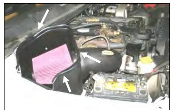
**9.** Install the Airaid Premium Filter (#1) onto the Intake tube as shown and tighten the clamp. Install the Weatherstrip (#6) onto the top edge of the CAB starting from the front and work your way back
