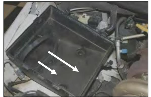
**3.** Locate the fender air scoop inside of the factory air box and remove it by pulling outward. The remaining factory airbox half can now be removed by simply pulling upward and off of the mounting studs on the inner fender well.
