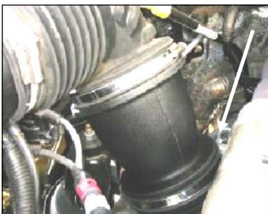
**7.** Install the Airaid Intake Tube assembly onto the turbocharger inlet. Tighten the factory hose clamp.
