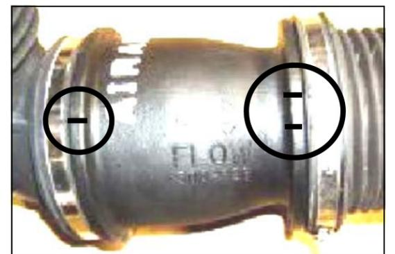
**6. Note:** Each side of the Airaid Intake Tube has notches that must be aligned with the notches on the factory intake tubes. Also, the flow arrow must point down towards the turbocharger inlet.
