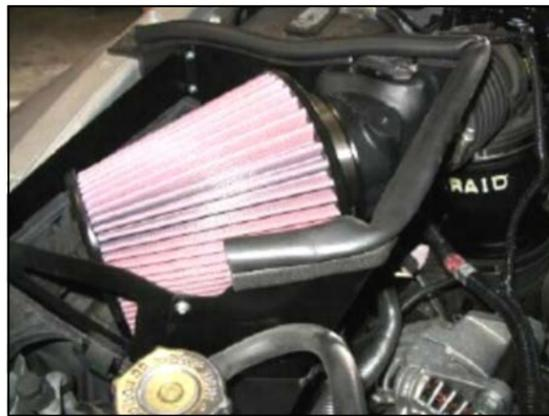
14. Install the Airaid Premium Filter (#1) onto the air filter adapter, and tighten the clamp. Install the weather strip (#6) onto the top of the **CAD**. (Hint: start at one end, and work to the other).
