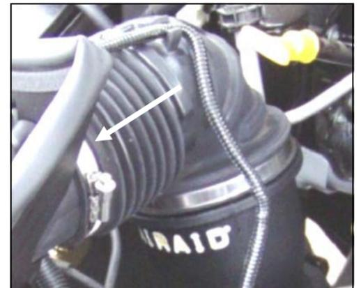
12. Slip the intake tube onto the air filter adapter, and tighten the clamp.
