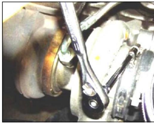
**2.** Using a 7mm socket, loosen the hose clamp where the factory intake tube connects to the turbo housing.
