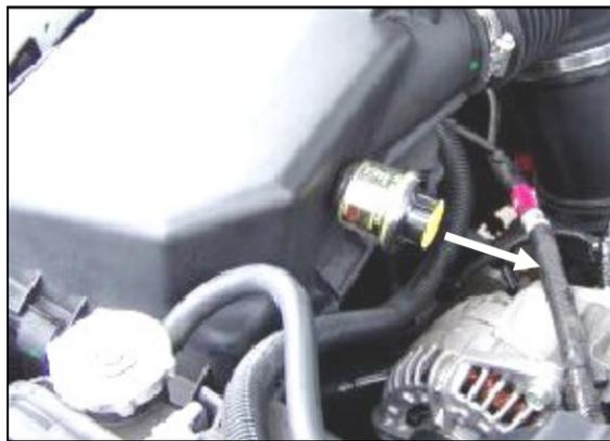
2. Remove the factory filter minder and rubber grommet (save for reuse).
