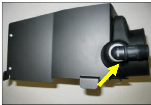
**5.** Install the supplied nylon fitting into the air filter adapter as shown.
