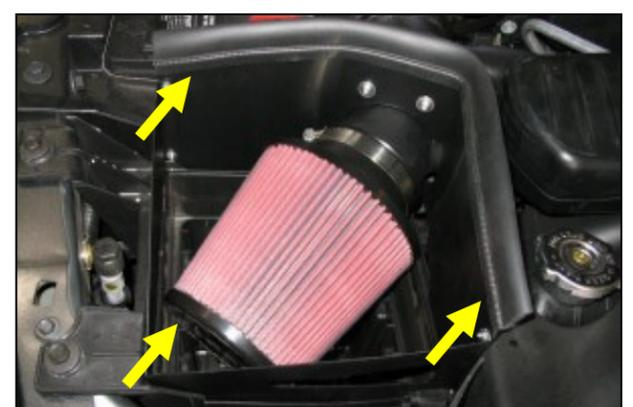
**9.** Install the Airaid Premium Filter on the end of the air filter adapter, and tighten the hose clamp. Install the supplied weather strip on the Cool Air Dam. (Note: start from one end and work your way around to insure proper alignment of weather strip.)
