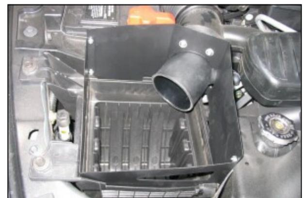
**6.** Install the Airaid Cool Air Dam assembly on top of the factory air filter base. Reconnect the factory intake tube, and tighten the hose clamp.
