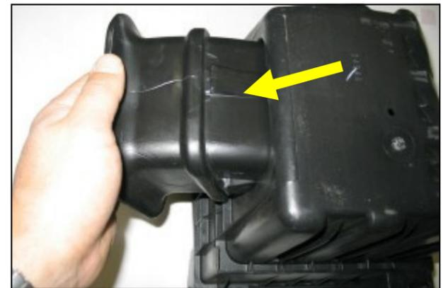
**3.** Using a 13mm socket, remove the air box base from the engine compartment. Using a flat blade screwdriver, carefully unsnap the box inlet from the base and remove it. Reinstall the factory base in the engine compartment without the inlet.
