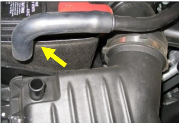
**1. Disconnect The Negative Battery Terminal!** Disconnect the factory breather hose and remove from the vehicle. (Note: 4.7L engines require the removal of the breather hose end section only. 5.7L Hemi required removal of entire hose assembly.)
