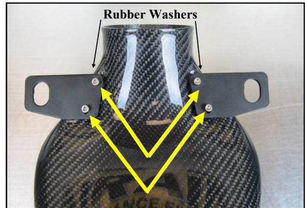
2. Set the Rubber Washers (#8) onto the Intake Tube and align with the threaded holes of the inserts.
