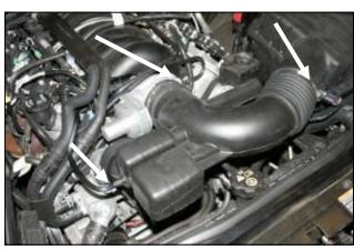
2. Disconnect the breather hose elbow by pulling it straight away from the intake tube. It is only held in place by an O-ring. Loosen the two hose clamps that secure the intake tube to the throttlebody, and the air box lid. Remove the air intake tube.
