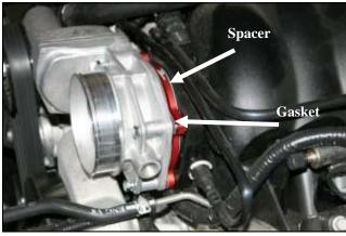
**4.** Install the Poweraid Spacer between the throttlebody and the intake manifold with the supplied gasket next to the throttlebody as shown. \*Note: Poweraid spacer must be installed with bore protruding into intake manifold away from throttle body. Incorrect installation will hinder performance. Reference picture below for spacer orientation.
