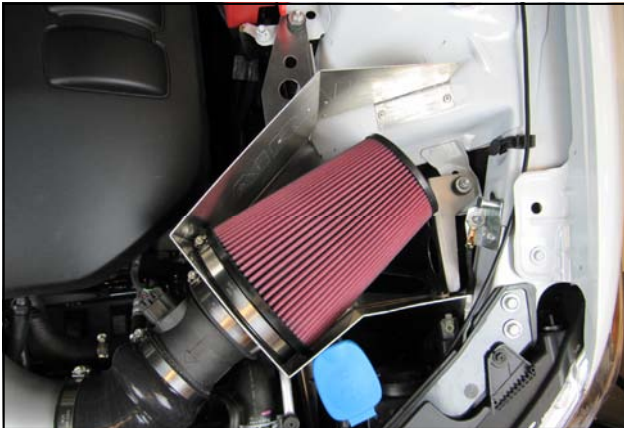
19. Install the Airaid Premium Filter on to the Filter Adapter.
