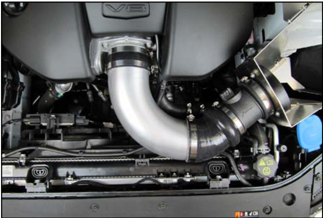
17. Slide the Intake tube into the Hump Hose first, then into the Coupler. Check the positioning of al the components. Adjust if necessary and tighten the Clamps.
