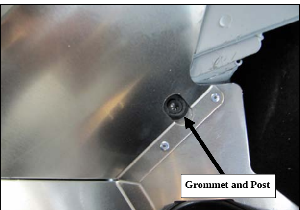
12. The bottom of the Air Dam assembly is to be secured using the grommet and post. Re connect the intake tube to the Mass Air Flow meter and reinstall the battery post cover.
