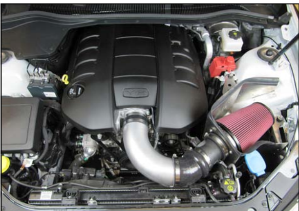
18. Reconnect the Air Flow Meter and reinstall the Positive terminal cover removed in step 1.
