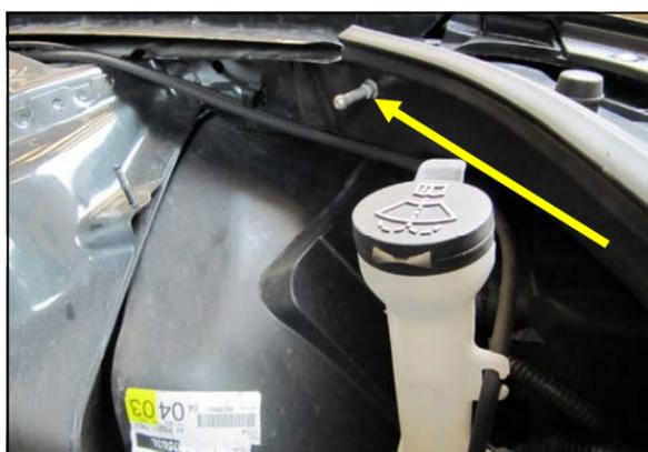
**8. Remove and save the ground lug from the driver's side inner fender.** It will be re-used in step #11.
