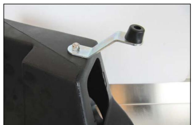
**6. Turn the Box upside down and mount the Lower Bracket (#10) using the 1/4-20 x 3/4" Hex Bolt (#16), 1/4" Flat Washer (#18), and 1/4" Nylon Lock Nut (#20) as shown. Attach the Plastic Bumper (#11) to the Bracket using the 8-32 x 5/8" Button Head Screw (#24), and the #8 Kep Nut (#25).**
