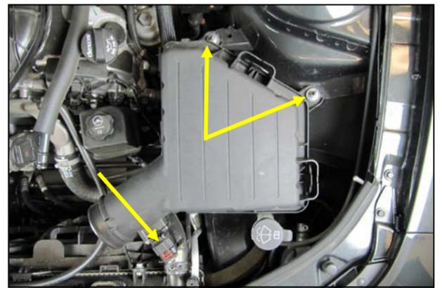
**3. Disconnect the Mass Air Flow sensor.** Using a deep 10mm socket, remove and save the two nuts that secure the factory airbox to the inner fender. These will be re-used in step 10. Lift up and remove the entire airbox and scoop assembly.
