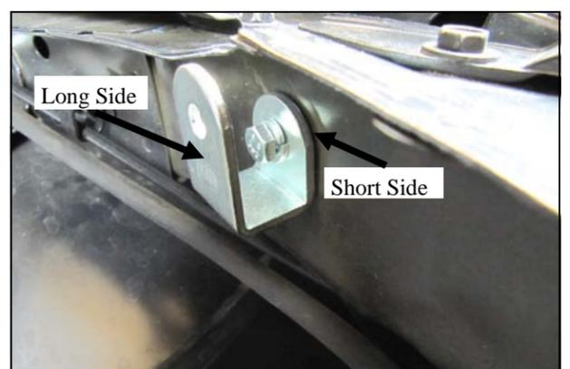
**9. Install the Side Bracket (#12) where the ground lug was installed, using the 6mmx12mm Hex Bolt (#21), and Lock Washer (#19).**
