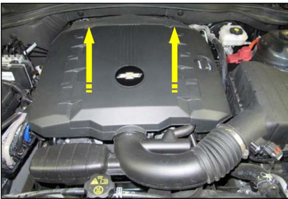
**1. Disconnect The Negative Battery Terminal.** Remove the oil fill cap and then lift up on the front of the engine cover to remove it from the vehicle. Replace the oil cap to make sure nothing falls into the motor during the install.
