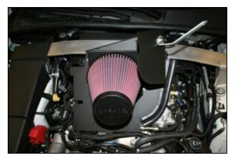
**10.** Install the Bracket (#27) on to the Rear Panel (#4) as shown using one 1/4-20 Button Head Screw (#19), 1/4" Flat Washer (#18), and 1/4" Serrated Nut(#20). Complete the assembly by attaching the Airaid Premium Filter (#1) to the Filter adapter (#8).
