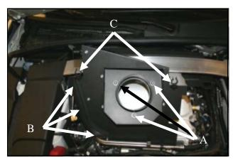
**8. A)** Install the Filter Adapter onto the MAF panel using three 1/4-20 Button Head screws (#17) and 1/4" Flat washers (#18). **B)** Attach the Weather Strip (# 11) to the curved edge of the MAF Panel. **C)** Insert the 5/8" hose anchors (#29) into the two horizontal tab holes on the MAF panel
