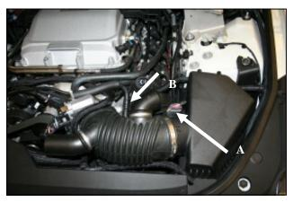
**2. A**) Disconnect the Mass Air Flow (MAF) sensor. B) Disconnect the PCV breather line by depressing the 2 Grey buttons in the fitting and pulling. Loosen the clamps securing the intake tube to the throttle body and airbox and remove the factory intake tube.
