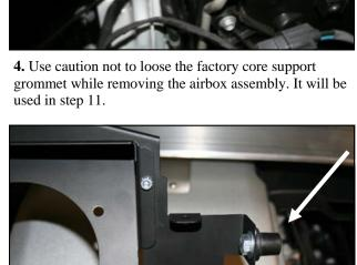
7. Attach the 5/8" Well Nut (#23) to the vertical MAF Panel tab as shown using the 5/16 Hex Bolt (#21) and the 5/16" flat washer (#22).
