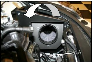
11. A) Locate and remove the Factory Ground strap bolt in the chassis. B) Lower the Airaid Performance Airbox assembly into the engine cavity. Insert the Well Nut into the Factory core support grommet and rotate the assembly rearward until the bracket rests on the shock tower and the MAF panel's lower tab hole is lined up with the Chassis bolt hole. Secure the assembly by
