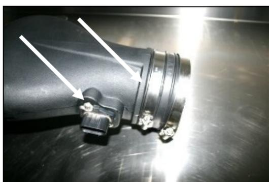
7. Reinstall the Mass Air Flow sensor removed in step #4, into the Airaid Intake Tube using two 8-32x3/8" button head bolts (#7).
