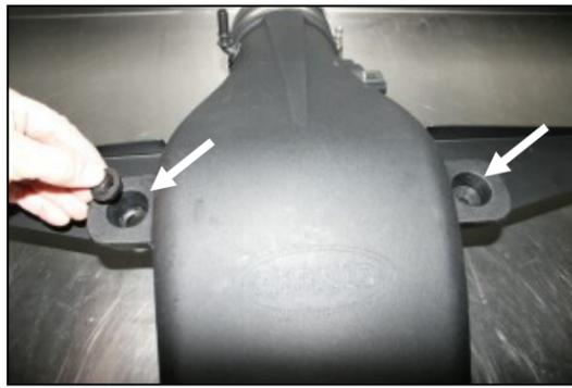
11. Install the provided grommets (#15), narrow side down, into the Airaid Intake Tube as shown. Make sure that they are seated all the way into the bottom of the holes.
