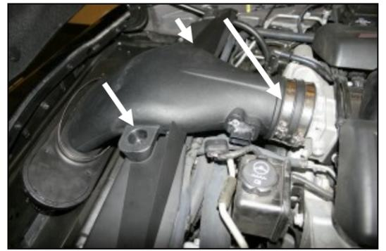
12. Install the Airaid Intake Tube assembly onto the throttle body first, and then align the grommets over the factory grommet posts on top of the radiator shroud. Push down on the grommets to seat them on the posts. (Hint: Use a 1/2" deep socket to help seat the grommets onto the posts.) Now tighten the hose clamp on the throttle body.
