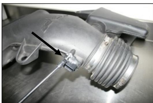
4. Using a #20 Torx Bit, remove the two factory screws that hold the MAF sensor into the factory intake tube. Remove the MAF sensor for reinstallation in step #7.
