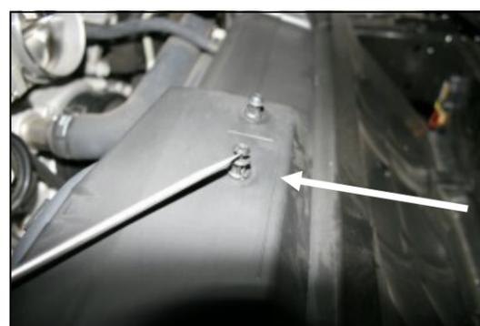
9. Using a flat blade screwdriver, pry up the center pin in the grommet post closest to the right fender on the radiator shroud, and remove both pieces of the grommet post from the vehicle.
