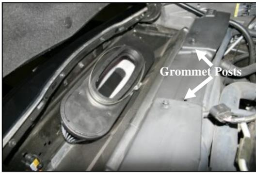
10. Set the Airaid Premium Filter into the area in front of the radiator. It will be mounted in step # 15.
