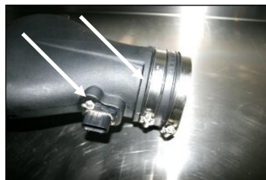
9. Reinstall the Mass Air Flow sensor removed in step #5, into the Airaid Intake Tube using two 8-32x3/8" button head bolts (#7).
