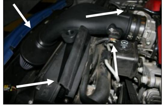
15. Slide the Airaid Premium Filter up onto the end of the intake tube and tighten the clamp. Reconnect the MAF sensor wiring harness and replace the grey security clip. Reconnect the factory breather hose to the breather fitting. Install the weather strip (#6) onto the top of the air dams as shown.
