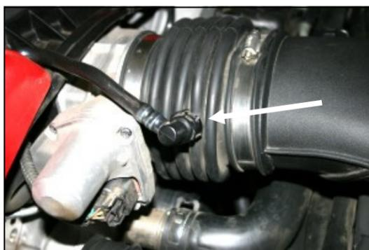
2. Push the tab on the top of the crankcase breather connector, and disconnect the breather hose from the factory intake tube breather fitting.
