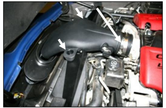
12. Install the Airaid Intake Tube assembly onto the throttle body first, and then align the grommets and the holes in the air dams over the factory grommet posts on top of the radiator shroud. Push down to seat the grommets on the posts. Now tighten the hose clamp on the throttle body.
