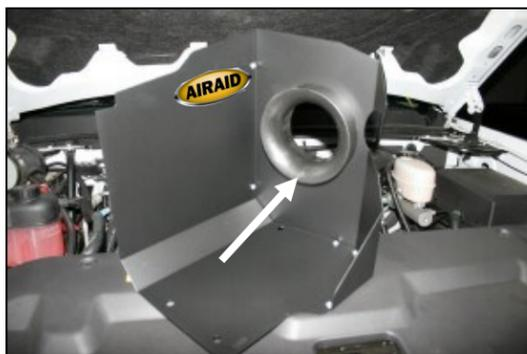
8. Assemble the Cool Air Dam panels (CAD) (#2 & #3) using five 6-32 x 5/16" screws (#10), #6 flat washers (#11), and 6-32 keps nuts (#12). Next install the air filter adapter (#5) into the panels as shown using three 1/4 - 20 x 1/2" button head bolts (#13), and 1/4" flat washers (#14). Apply the Airaid Foil Decal onto the Panel as shown.
