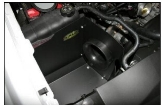
9. Install the Airaid CAD assembly into the vehicle replacing the factory airbox. Secure the CAD using four M6 x 1.25 Hex Bolt (#15), and 1/4" flat washers (#14). Do not over tighten the four bolts.
