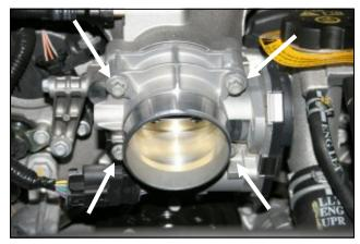
**3.** Remove the four bolts that secure the throttlebody to the intake manifold. *Note that the lower passenger side bolt secures a metal bracket holding a wiring connector. Make sure to remount this bracket in the same location in step #4.*
