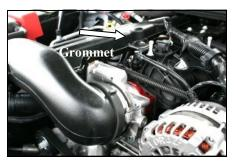
9. Re-install the intake tube using caution to center the intake tube hole over the previously installed grommet. Some adjustment may be required to seat the grommet correctly back into the intake tube. Tighten the hose clamps on the tube. Re-connect the breather tube. Re-install the plastic holder from step #1. Re-install the beauty cover. Re-connect the negative battery cable!
