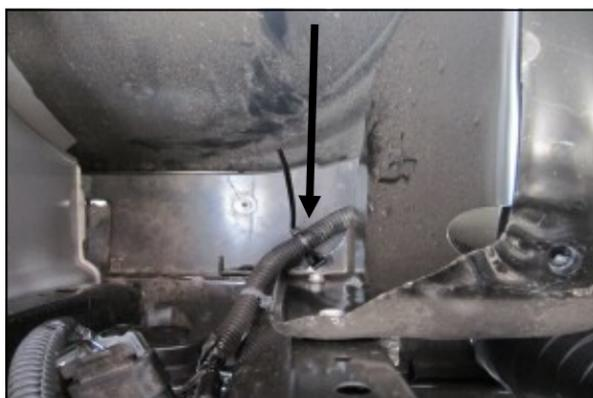
8. Secure the wiring harness to the inner fender as shown using the Edge Clip Cable Tie (#15).
