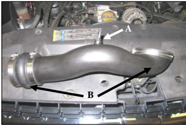
11. A.) Install the 3/8 NPT Fitting (#14) in to the Airaid Intake Tube.
