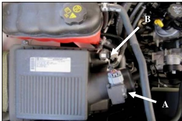
5. Disconnect the Mass Air Flow or MAF sensor ( A ) and the Manifold Absolute Pressure or MAP sensor ( B ) Remove the factory airbox from the vehicle. The airbox is secured to the vehicle with grommets and simply lifts out.
