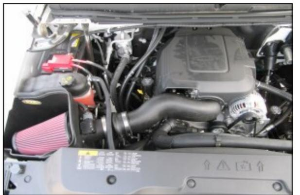
15. Reinstall the engine cover. Double check your work! Make sure there is no foreign material in the intake path. Make sure all clamps, hoses, bolts, and screws are tight. Double check the hood clearance. Reconnect the negative battery cable.
