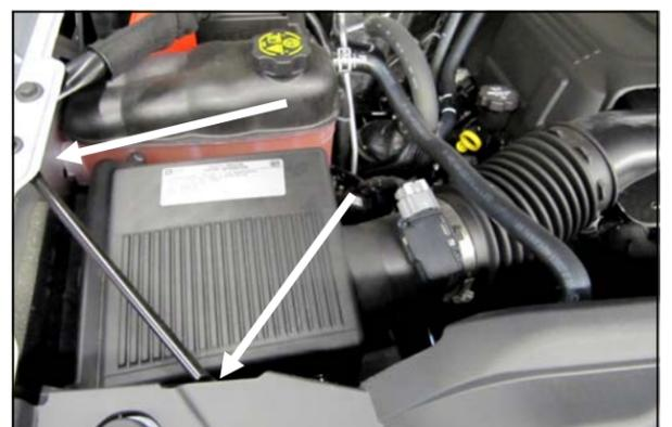
6. **On 2015 Models:** Remove the two 6mm bolts in the fender brace and set the bolts and brace to the side.
