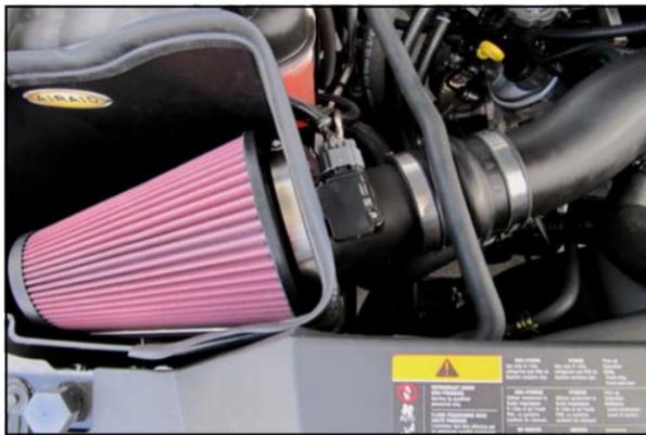
14. Install the Airaid Premium filter (#1) onto the Filter Adapter, and tighten the hose clamp. Reconnect the MAF And MAP sensors. Install the Weather Strip (#8) onto the Airaid Cold Air Box. (*Hint: Start from one corner and work your way around for ease of install.*)
