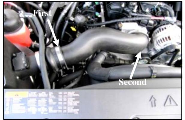
12. Install the Airaid Intake Tube assembly onto the Filter Adapter first, and then onto the throttlebody. Adjust for fit, and tighten all hose clamps. Reinstall the hose anchor into the Airaid Intake Tube.
