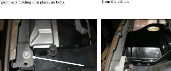
7. Remove the factory bolt that secures the right front fender to the radiator support. It will be reused in step
