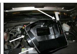
6. Install the filter adapter (#4) into the Cool Air Box (#3) as shown using three 1/4" Button head bolts (#8) and three 1/4" flat washers (#11). Next, fasten the bracket (#15) to the front of the CAB as shown using one 1/4-20 hex bolt (#9) two flat washers (#10), and one 1/4" Nylock nut. Refer to the drawing above for reference.
