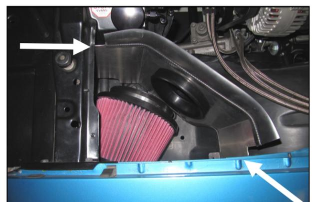
**6. Carefully install Air Dam assembly in to the inner fender area. Note-The outermost edges will be underneath the core support and the fender when installed**
