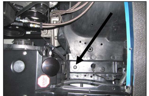
**3. Driver Side - Remove the inner fender bolt and set it aside. It will be re used in step #7. Passenger Side - Remove the battery and tray if not already relocated. One of the Tray bolts will be re used in step #7.**
