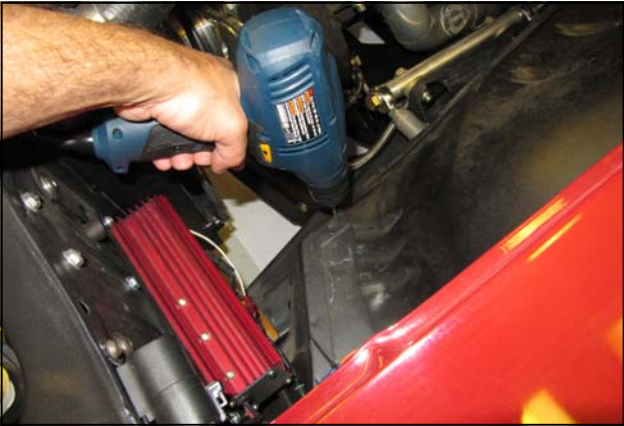
10. Drill 1/8" pilot holes into the inner fender.
