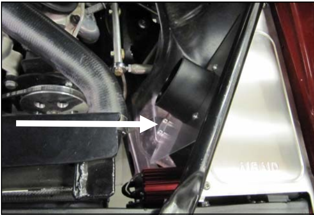
13. Secure the Air Dam tab to the inner fender using the two Self drilling screws (#8).
