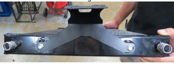
94. Back out the four (4) crash beam bolts (circled in image) but do not remove. Install the LTR assembly from under the crash beam and onto the crash beam support studs. Line up the holes on the LTR brackets with the studs to temporarily hold the LTR in place for the next step.
