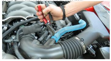
31. Remove the brake aspirator hose from the air inlet tube.
