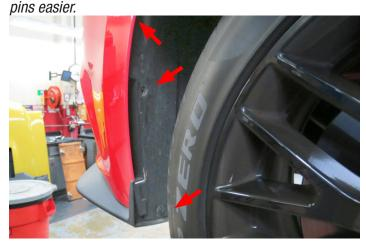
23. There is an additional push pin located just above the tire that needs to be removed.
