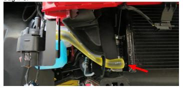
101. Insert the LTR to Manifold hose through the hole on the upper shroud and secure to the top LTR bung with a hose clamp from Bag # 3. Secure the other end to the lower bung on the supercharger manifold.
