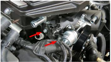
71. Using O-ring lube, install the fuel rail fittings onto the fuel rails. The passenger side rail will have the black plug on the front of the rail, while the driver will have the 180° fitting. Attach the supplied fuel crossover to the rear of both rails.
