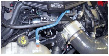
87. Carefully remove the protective foam from the brake aspirator.
