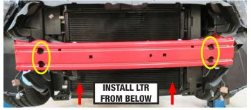
95. Install the supplied beams using the two (2) M8 x 30mm hex flange bolts from Bag # 3, loosely screw in the bolts through the crash beam braces. The lower crash beam braces will sandwich the LTR to the crash beam and be secured using the M8 nuts and washers supplied in Bag # 3. Once all bolts are in place through the braces, fully tighten the bolts and nuts.
