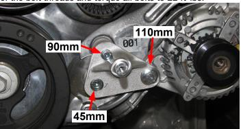
58. Install and secure the 76mm idler pulley onto the center of the idler bracket by using the M8 Washer and the M8 x 20mm bolt supplied in Bag # 3 using a 12mm socket. Use blue thread lock fluid on the bolt threads and torque to 18 ft-lbs.
