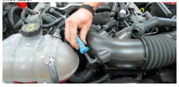
34. Disconnect the brake aspirator hose from the manifold PCV hose.
