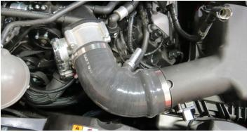
123. Connect the brake aspirator to the lower fitting on the silicone elbow.
