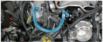
41. Disconnect the throttle body connector.
