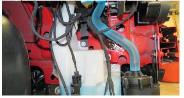
104. Secure the Surge Tank to Manifold hose to the surge tank and manifold using two (2) hose clamps from Bag # 3.
