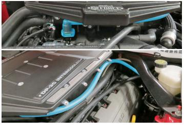
111. Connect the supplied straight quick connect fitting on the EVAP hose to the hard line.
