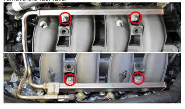
47. Using an 8mm socket, remove six (6) manifold bolts.
