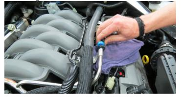
46. Using a 10mm socket, remove four (4) bolts securing the fuel rail and manifold. *TIP:* It's not required to fully remove the fuel rails.
