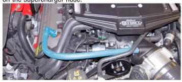
109. Using a razor blade, remove the 90° fitting on the factory EVAP hose.
