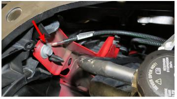
118. Attach the overflow hose onto the top barb of the surge tank and route the end of the hose towards the ground on the side of the water pump. **NOTE: Loosley secure the end of the hose to another existing hose or chassis and ensure that the end of the hose is never close**
