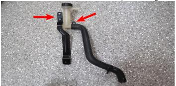
103. Connect the Water pump to Surge tank hose to the water pump and secure with a hose clamp from Bag # 3.
