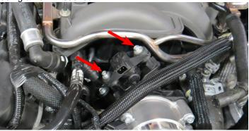
70. Install the EVAP solenoid to the supercharger manifold using two (2) M6 x 25mm bolts in Bag # 1.
