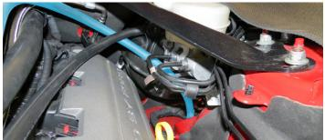
112. Zip tie the Fuse holder on the "Water Pump/EVAP Harness" onto the top right corner of the fuse box.
