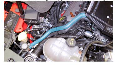
105. Attach the surge tank to the surge tank bracket using two (2) M6 x 10mm bolts from Hardware Bag # 3.
