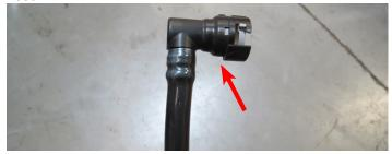
108. Attach the 90° fitting onto the supplied 1/2" Cadbar hose. Connect the quick connect fitting to the passenger side valve cover and the other end of the hose to the barb on the supercharger nose.
