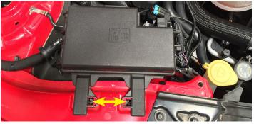
116. Mount the Relay on the "Water Pump/EVAP Harness" below the fuse box and secure it with the Push Pin supplied in Hardware Bag # 3. Once the Relay is mounted, resecure the Fuse box.
