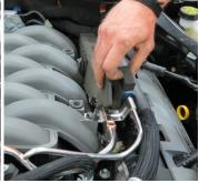
44. Disconnect eight (8) fuel injector connectors.
