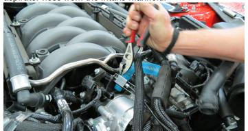
38. Remove the brake aspirator hose assembly from the brake booster and set aside as it will be reused later.
