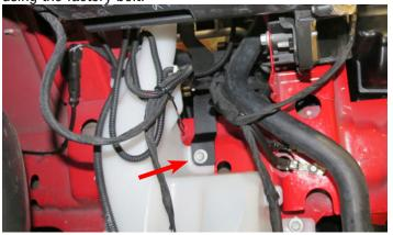
107. Using a razor blade, or equivalent, remove the 90° quick connect fitting on the factory passenger side PCV hose.
