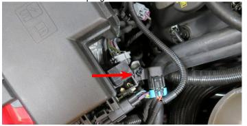
113. Open the fuse box and using a 10mm socket, attach the "Power Supply Wire" of the "Water Pump/EVAP Harness" to the power terminal on the fuse box.
