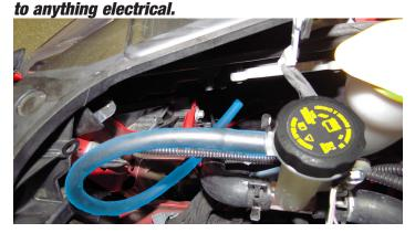
119. Connect the factory EVAP connector onto the "Engine Harness" end of the "Water Pump/EVAP Harness" and the "EVAP Solenoid" end onto the EVAP solenoid.
