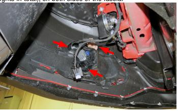
26. Tape up the fender as needed to prevent scratching the painted surfaces. With the help from an assistant, carefully disengage both sides of the fascia by gently pulling the sides outwards. Remove the fascia and set aside.
