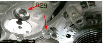
57. Secure the idler bracket by installing bolts from Bag # 2. The M10 x 110mm bolt through the ear of the alternator, the M8 x 90mm bolt into the top front cover hole, and the M8 x 45mm bolt through the lower hole that was used to secure the stock tensioner. Use blue thread lock fluid on all of the bolt threads and torque all bolts to 22 ft-lbs.
