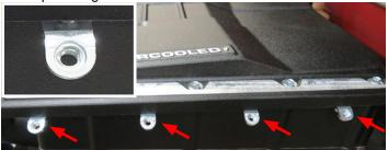
68. For proper bracket alignment, test fit the side covers onto the brackets using eight (8) M6 X 25mm bolts from the side cover kit. While pushing the side covers forward, fully tighten the bracket bolts. Once all brackets are aligned and tightened, remove the side covers.
