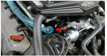
84. Use a 3/8" breaker bar to rotate the tensioner clockwise, finish installing the supplied belt according to the routing diagram shown below.
