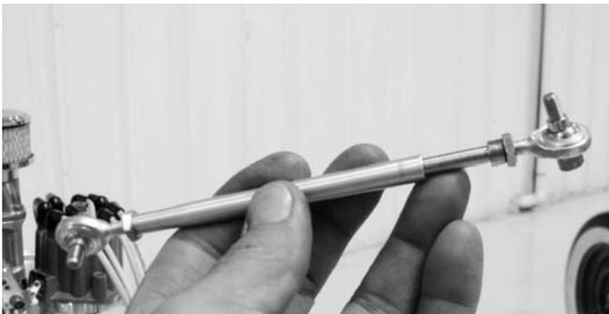
1. Install secondary linkage between the front and rear carb as in steps 1-3 above.
