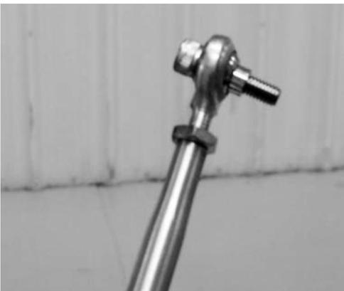
3. Install linkage end on lower hole of throttle arm on both carbs by inserting the bushing through hole in throttle arm and secure with washer and locknut.
