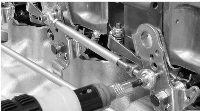
3. Connect slider link to the upper threaded hole in center carb throttle arm, connect other end of slider link to the lower threaded hole in the rear carb throttle arm.
