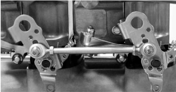
5. With throttle blades of both carbs closed adjust the link length so that both carbs hit the idle stop screw at the same time. Tighten rod end jam nuts. Back off idle speed screw of the front carb 2-3 turns. Engine idle speed adjustments will now be made at the rear carb. Start engine and proceed with carb adjustment and synchronization.
