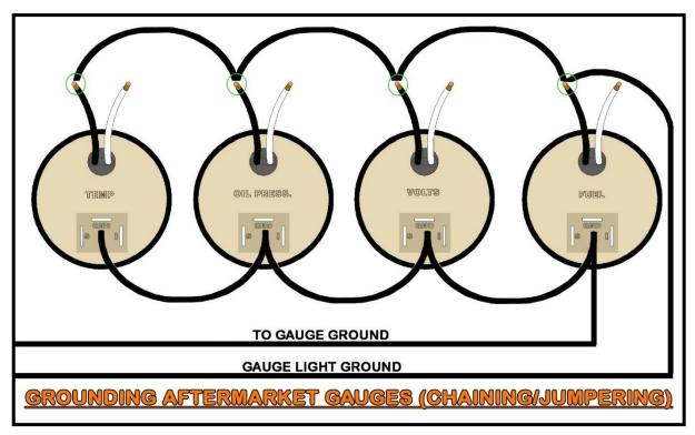
Gauge light power is supported by the **BROWN #930** wire. This wire connects to one of the leads for the gauge light or to the gauge light tab found on gauges with LED backlighting. To make these connections you can splice from this **BROWN #930** wire to all the gauges or chain/jumper it all together.
