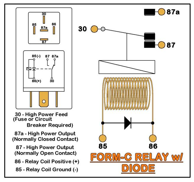
This kit is supplied with a diode suppressed, weatherproof relay. This diode prevents the back-feeding of residual coil energy and voltage spikes when the coil is deactivated.
