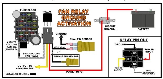
IN THE EVENT THAT A TOGGLE/ROCKER SWITCH IS BEING USED WITHOUT A RELAY, MAKE SURE THE AMPERAGE OF THE COMPONENT YOU ARE POWERING DOES NOT EXCEED THE CAPABILITIES OF THE SWITCH OR SWITCH FAILURE WILL OCCUR. IF YOU NEED A RELAY KIT PAINLESS OFFERS PART #'S 30128, 30128, & 30130.
