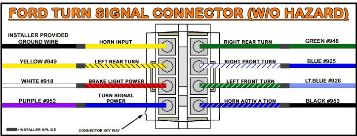
The diagrams above show splicing the wires from the Painless harness to an installer created pigtail from factory wiring.
