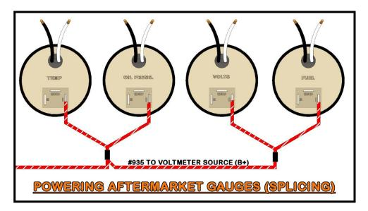
**#2)** Chaining or Jumpering- Run the RED/WHITE #935 wire to a power post. Before terminating the wire with the proper terminal, insert another wire into the terminal and crimp. You now have 2 wires in 1 terminal. This additional wire then routes to the next gauge's power post. Before terminating that wire with the proper terminal, insert another wire into the terminal; and so on.
