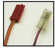
Using the terminal removal procedure, found on page 6, remove the two fuse block connectors on the factory harness. Remember to pry the locking tang of the terminal back out once the connector is removed. The factory connectors can also be cut from the original harness and the new terminals that are provided with the Painless kit can be installed.
