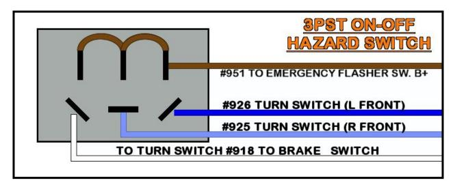
Also, a simple SPST On-Off switch can be used to flash only the brake lights in the event of an emergency. This diagram will not flash the front turn signals like a traditional hazard flasher which your local laws may require.
