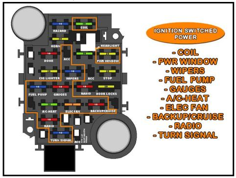
The drawing above shows all the switched ignition fuses. These fuses are powered by wires coming from the ignition switch (wires #931, #932, and #933) and receive power depending on what position the ignition switch is in. NONE OF THESE FUSES SHOULD HAVE POWER WHEN THE IGNITION IS IN THE OFF POSITION. The Ignition Switch Section beginning on page 89 of this manual will go into further detail about power supplied to these fuses.
