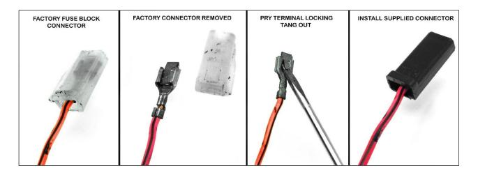
Install one of the single-pin connectors on each of the factory wires and connect them
