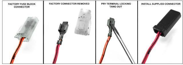
Install one of the single-pin connectors on each of the factory wires and connect them to the Painless harness. The factory pink/black wires connect to the power window, YELLOW #911 wire on the Painless harness. The factory, orange/black wire connects to the power lock, YELLOW/BLACK #910 wire on the Painless harness
