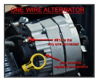
RED: 14-gauge wire, printed [ENGINE SECTION] #995 ALT. REGULATOR POWER (BATTERY), this is the sense wire, it provides a battery power source, or voltage sense, that all voltage regulators require. This wire has power at all times and comes from the large battery supply splice in the harness. This wire will not be needed if you have a one wire alternator or a GM CS series alternator. See the various alternator illustrations on pages 51 - 62 and the Charge/Battery Power Schematic on page 47.
