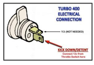
• If you have a factory, accelerator pedal mounted switch, you can use a switched power source inside the vehicle or you can route the cutoff piece of **#954** to the interior, connect at the throttle switch, and then route it back out to the transmission.
