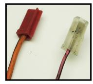
Using the terminal removal procedure, found on page 6, remove the two fuse block connectors on the factory harness. Remember to pry the locking tang of the terminal back out once the connector is removed. The factory connectors can also be cut from the original harness and the new terminals that are provided with the Painless kit can be installed.
