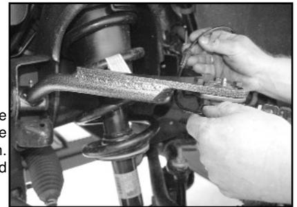
Route the factory ABS line and Attach the bracket to the stud on the new upper arm. Plug line back together and attach to factory clips.
