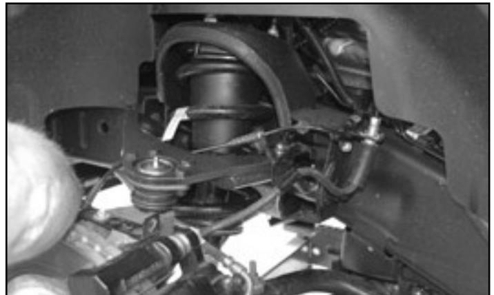
Measure completed height of vehicle and record on installation helper.
