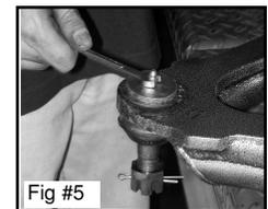
Install these control arms just like factory arms. Check your vehicles service manual for specific details. The arms can be installed in any order, lowers first than upper or upper than lower. DJM recommends installing one side at a time and complete the installation of either the upper or lower before starting on the next.
