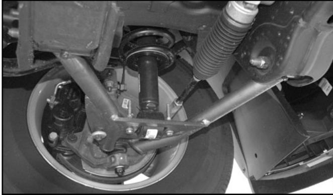
Check frame mounts for any dirt or debris. Test fit arm into frame mounts. They should slide in fairly easily. If they are too snug separate the mounts slightly. Install and grease fittings in the arm and ball joint. Apply some grease to the mounting brackets and the bushings. Install with factory bolts. See photo below for correct orientation of new arm.
