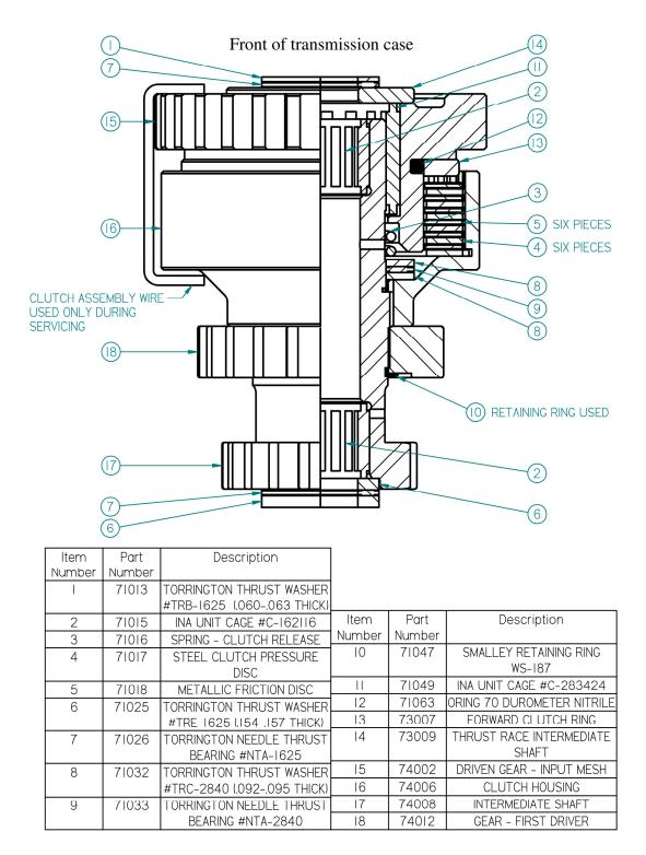
Figure 3. Clutch assembly with retaining ring (71047).
