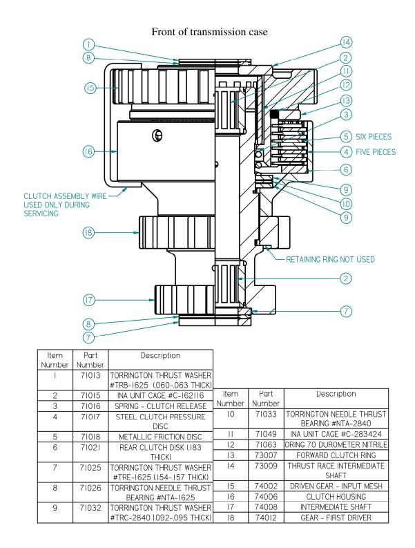
Figure 2. Clutch assembly without retaining ring (71047).
