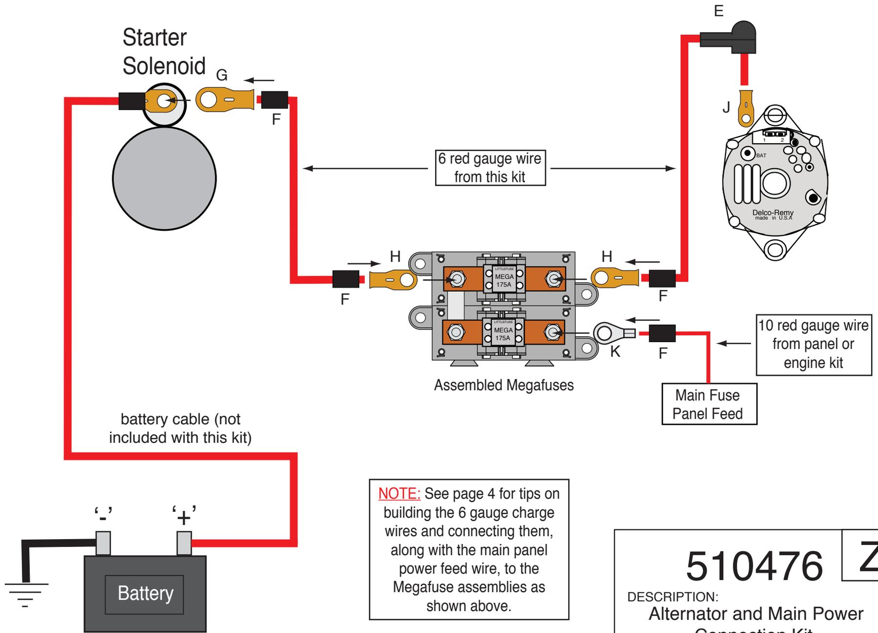
**NOTE:** See page 4 for tips on building the 6 gauge charge wires and connecting them, along with the main panel power feed wire, to the Megafuse assemblies as shown above.
