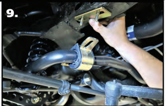
9. Install the bushing strap over the swaybar bushing with the wide side of the strap to the inside on the car. We found some steering box conversions hang down further than others. If yours happens to hit the sway bar, add a 2nd spacer under the bushing. a 2nd set of spacers along with longer hardware is supplied in this kit.
