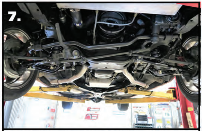
7. Insert the new swaybar from the passenger side. position it above the idler arm and steering arm. the center of the bar should hang down towards the ground.
