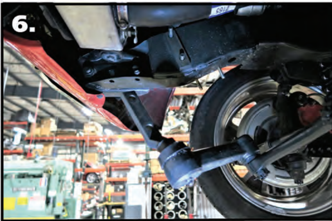
6. Disconnect the idler arms from the frame.
