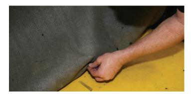
Be sure to trim any necessary shifter access holes - and route any electrical wires - before gluing down the rear half of the carpet.
