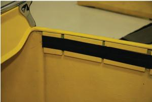
The side and back panels are secured to the body using the supplied hook-and-loop material. One side of the material is already attached to your panels; the other will need to be attached to the wood support pieces. Two 1" strips are applied approximately 1" below the body flange as shown.
