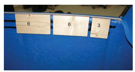
The wood blocks can then be attached. You may need to use clamps to temporarily hold them as the adhesive sets up. Start with a 3" block placed approximately 1" behind the dash, and then two 6" blocks behind it. Each block should be spaced about ½" apart.
