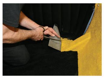
The rear half of the carpet can then be glued down in the same manner as the front. On channeled-floor bodies, you will need to trim out small pieces to clear the frame kick up as shown.
