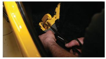
After attaching the side panels, you can trial fit the floor carpet. Before gluing the carpet down, you will need to trim a small access opening for the brake pedal.
