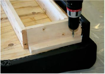
If you are building a T with an un-channeled body, you will probably want to use the supplied seat riser under your seat cushion. It can be attached to the seat bottom using  $1\frac{1}{2}$ " wood screws. Channeled cars will not need this riser.
