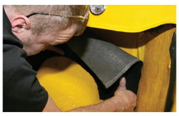
The carpet for the firewall comes trimmed to fit, but it's a good idea to trial fit it in your car before gluing. This will allow you to make any additional alterations that may be necessary.
