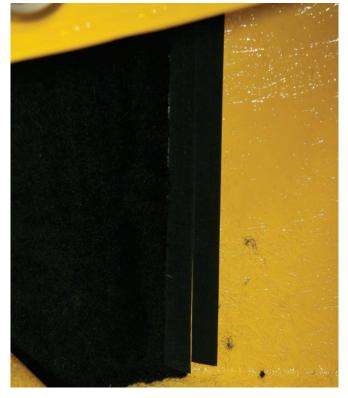
You will also need to put vertical strips of hook-and-loop material at the front of the body, right next to the corner of the firewall. This will support the front edge of the side panels.
