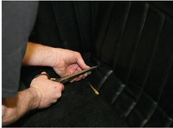
The seat back section is installed in the same manner as the side panels. You may need to make a couple of relief cuts on the bottom for the panel to fit flat on channeled-floor cars.
