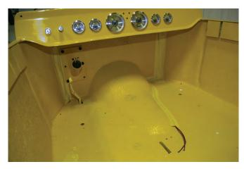
Before installing carpet, make sure all wiring is taped down as flat as possible where it runs along the firewall or floor.
