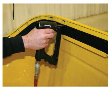
It's a good idea to use a staple gun to attach the hook-and-loop strips more securely, especially in the corners.
