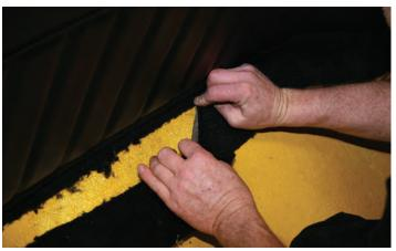
The carpet on the side panels is intentionally left long. Use a utility knife or razor blade to trim off the excess material where the side of the body meets the floor.
