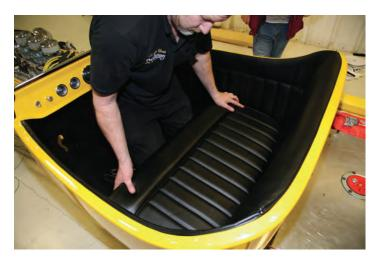
With the brace in place, the seat bottom can be installed in the car, completing your interior installation. The seat bottom is easily removed to provide access to the under-seat area.
