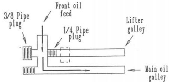
All threaded plug holes in blocks are National Pipe thread and use tapered pipe plugs. We recommend using female allen socket plugs. Various length plugs are available from Pioneer for adjusting the depth of the plug.
