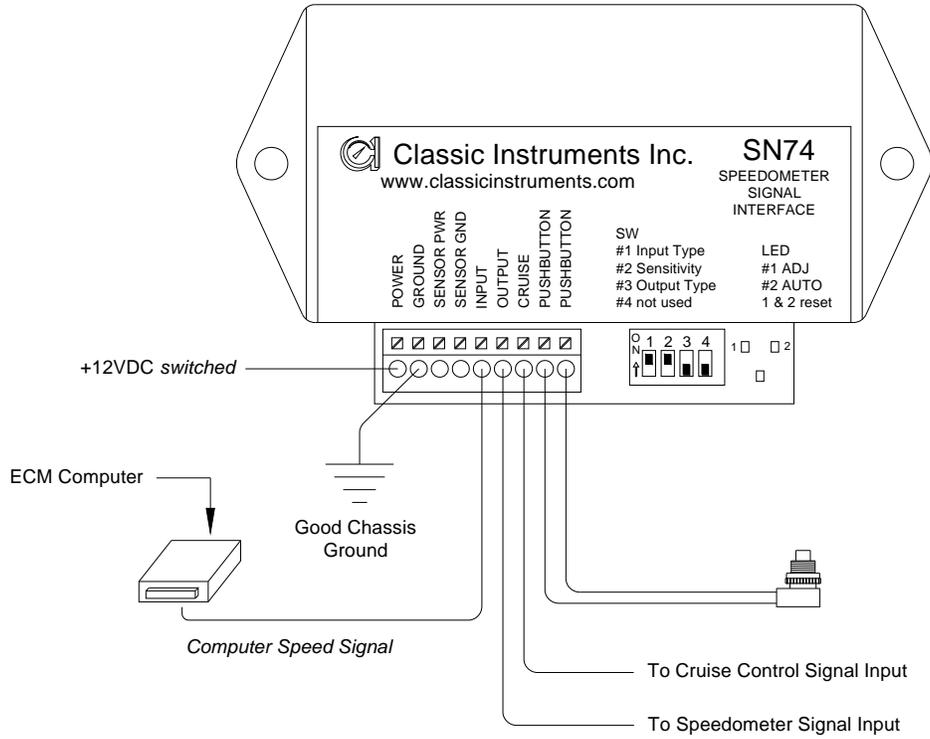
**Module Connected to ECM Speed Signal**
