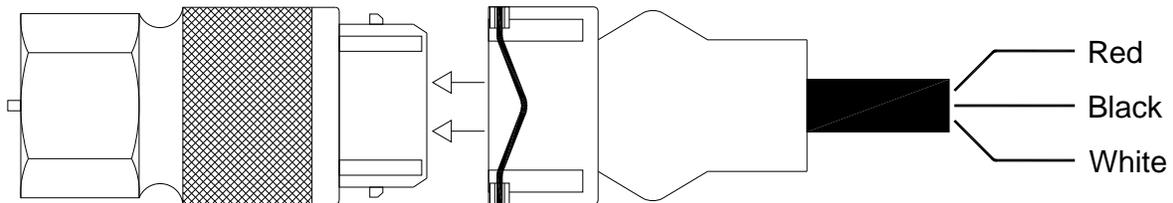
**Red:** +12VDC (to +12V terminal of speedometer)
