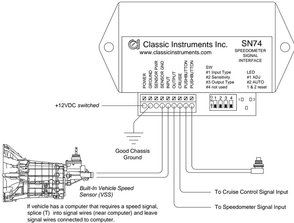
**Module Connected to Electronic Transmission's VSS**
