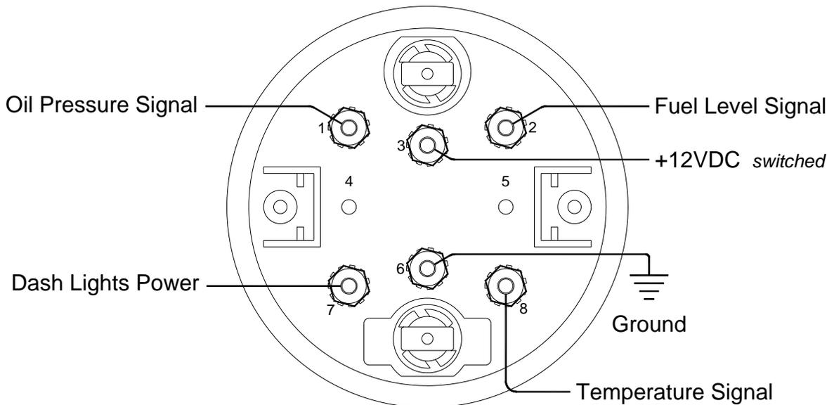
*Older 3-3/8" quad gauges have alternate labeling as follows: 3 = B+, 6 = GND, 8 = 3, 7 = 4*
