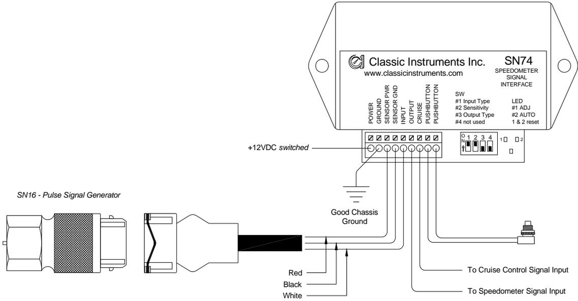
**Module Connected to SN16 Pulse Signal Generator**
