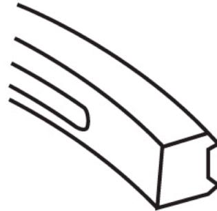
**CAST RINGS MUST BE INSTALLED USING A RING EXPANDER TOOL**
