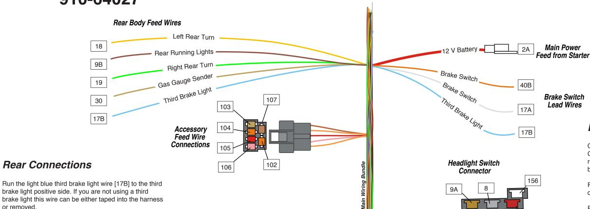
Run the light blue third brake light wire [17B] to the third brake light positive side. If you are not using a third brake light this wire can be either taped into the harness or removed.
