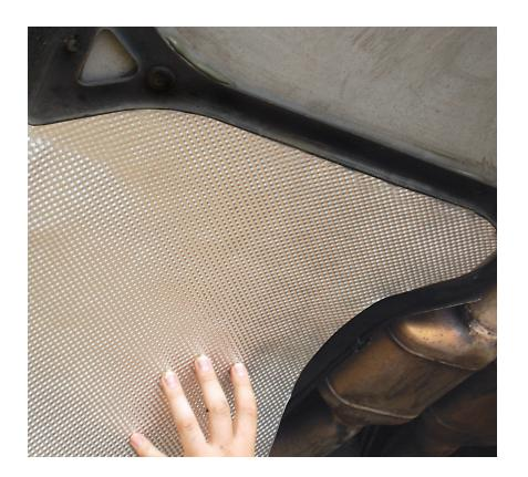
5. After Floor & Tunnel Shield II is set in proper location, apply pressure to ensure a strong bond with the installation surface.
