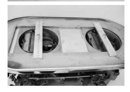
6. Install the filter element on to the base assembly and install the air cleaner top. Thread the two  $\frac{1}{4}$ "-20 x 2" flathead screws through the base and into the air cleaner top.
