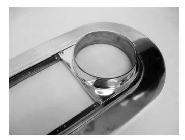
2. Position the front adapter on the carb. Position the rear carb adapter and base over the front carb adapter. Mark the position of the front adapter and remove from engine. Drill and tap four #10-24 holes to mount the front adapter to the base.
