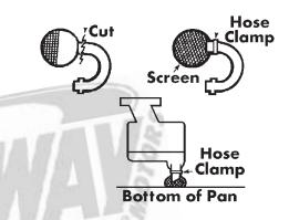
NOTE: We have available a prefabricated oil pump pick up designed to be used with our pan. 917-15135 for use with stock oil pump (OP55) 917-15136 for use with 4 bolt high volume oil pump (OP55HV)
