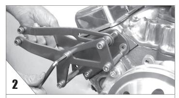
**INSTALL** the bracket to the head and snug up the bolts.
