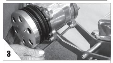
INSTALL the compressor by bolting to the bracket as shown.
