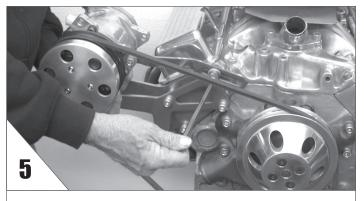
INSTALL the belt. Adjust tension and tighten the adjusting arm bolt. TIGHTEN all bolts, re-check tension and alighnment. Adjust as needed.
