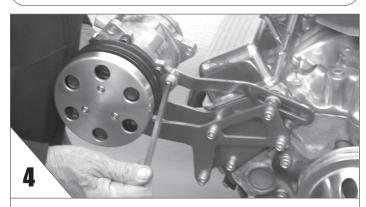
**BOLT** the adjusting arm to the compressor. Snug up the bolts.
