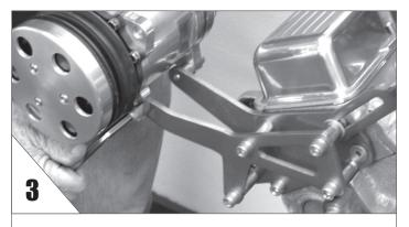
**INSTALL** the compressor by bolting to the bracket as shown, keeping the 5/8" spacer between the compressor mounting ear and the back plate.
