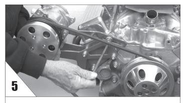
**INSTALL** the belt, adjust tension and tighten the adjusting arm bolt. **TIGHTEN** all the bolts, re-check tension & alignment. Adjust as needed.
