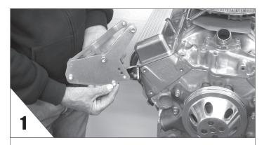
**REMOVE** the nut, plastic sleeves and tape from the bolts. **NOTE:** Please do not disassemble the bracket.
