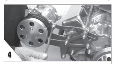
**BOLT** the adjusting arm to the compressor. Snug up bolts.
