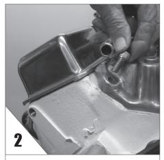
REMOVE the 1st intake manifold Bolt.
