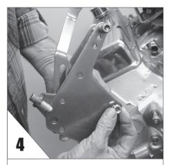
**REMOVE** nut, plastic sleeves and tape from the bolts! NOTE: Please do not disassemble the bracket!
