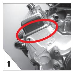
POSSIBLE VALVE COVER FLANGE TRIM-MING: A minor bit of trimming on the Valve Cover Flange (circled in red) may be needed to allow the bracket to sit flat on the head
