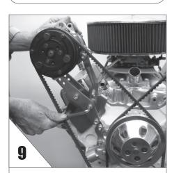
ADJUST the belt tension. Tighten up all bolts now and check for proper alignment.
