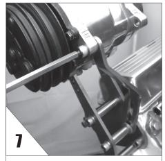
SWING the adjusting arm up and bolt it to the compressor. Snug up bolts for now, not tight.
