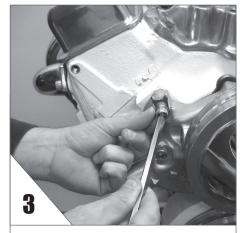
INSTALL the WPC (Water Pump Cradle) by removing the top water pump bolt. Leave slightly loose.
