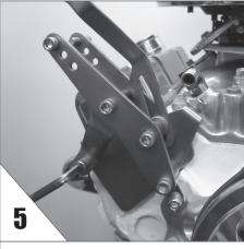
NOW BOLT the bracket to the head and snug up the bolts. THEN LAY the adjusting arm on the engine to get out of the way.
