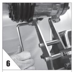
**INSTALL** the compressor to the bracket. Keep the 5/8" spacer between the back plate & rear compressor ear, & snug up.
