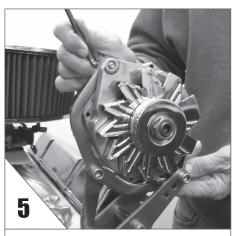
NOW SWING the adjusting arm over and hook the 'C' brace to the alternator bottom, then BOLT the top of the 'C' brace to the alternator as shown!
