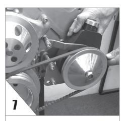
**TIGHTEN** all the bolts and install the belt. Adjust for tension, check that all bolts are tight and the pump is properly aligned.
