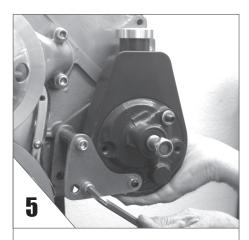
**BOLT** the pump to the block.
