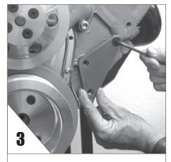
**BOLT** the spacer plate to the block.
