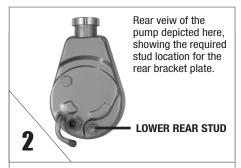
**LOWER REAR STUD** is required for installation.
