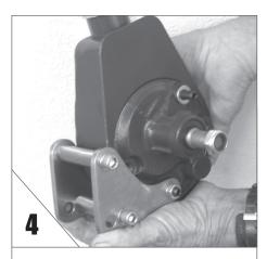
**ATTACH** the bracket to the pump as shown above.
